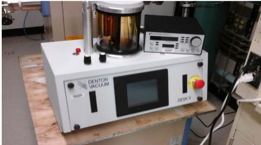
Figure 18: Denton Vacuum Sputter Coater
